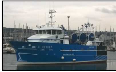
2 gensets 400 kVA high efficiency + 2 x 221 kW propulsion - Trawler
