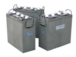
Optimum charge voltage depends on temperature. Typical values are 2.27V/element at 20°C and 2.25V/element at 25°C. For applications with high temperature variations, the adjustment of charge voltage is recommended. When housed in containers, the optimal place for taking the temperature is at 2/3 of the height, with the probe being placed in the centre at this level.
